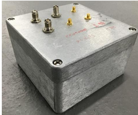
Figure 1 – Supplied enclosure with coaxial bulkhead connectors fitted
